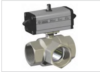
Ball Valve with DA Actuator Material: Brass Ports: 'L' & 'T' / Size Range: 3/8"-2" Pressure Range: PN 16
