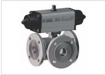
Ball Valve with SR Actuator Material: SS (Flanged Type) (Temp: 20 to 160°C) Ports: 'L' / Size Range: 3/8"-4" Pressure Range: PN16, 25, 40
