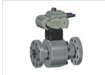
Split Body Valve with Electrical Actuator Material : SS / Size Range:1/2"-4" Pressure Range: PN63- 100 ANSI 600/900- 1500
