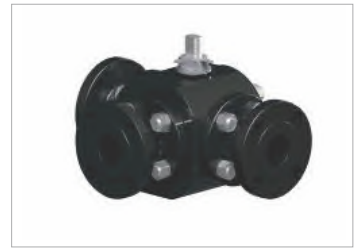
Thor Split Body 3 Way Material: CS & SS / Size Range: 1/2"-4" Ports: 'L' & 'T' ANSI 150 - 300 Pressure Range: PN16 - 40
