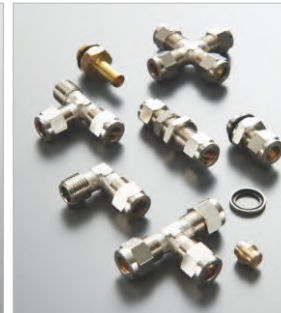
10000 Series( Universal Double Cone Fittings) Materials: Nickel Plated Brass Max. Press.: 128.6 bar Temp.: -60°C to +300°C
