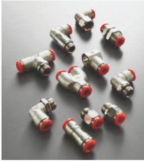
50000 Series with Red Collet Push-In Fittings Temp.: -20°C to +80°C Press.: -0,99 bar to 20 bar Fluids: Compressed Air, Vacuum
