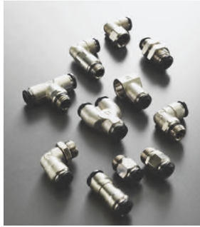
50000 Series with black Collet Push-In Fittings Temp.: -20°C to +80°C Press.: -0,99 bar to 20 bar Fluids: Compressed Air, Vacuum
