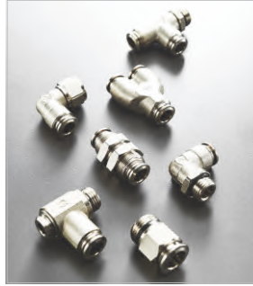
57000 Series Metallic Push-In Fittings Temp.: -20°C to +80°C Press.: -0,99 bar to 20 bar Fluids: compressed air, vacuum, water, steam (EPDM seal )
