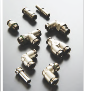
40000V Series Metallic Push-In Fittings with FKM Seal Specially for Steam Applications Temp.: -15°C to +130°C Press.: -0,99 bar to 20 bar
