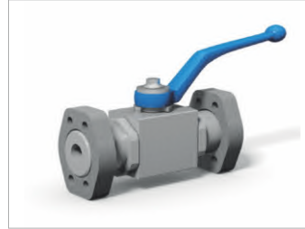
2/2 way ball valves with SAE connection. Pmax: 210-420 Bar. Size: DN13-125 Metric Thread, UNC thread
