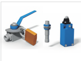
2/2 way ball valve with locking device safety against unintentional actuation / different types / tamper proof. Pmax:500 bar, Size: DN4-25/40
