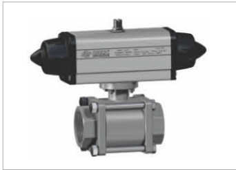
Three Piece Ball Valve with SR Actuator Material: Stainless Steel Size Range: 1/4"-4" Pressure Range: PN63
