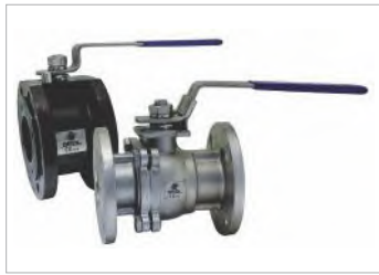
Casted Ball Valve Manual Version Material: CS & SS Size Range: 1/2"-4" Pressure Range: PN 16-40 / ANSI 150
