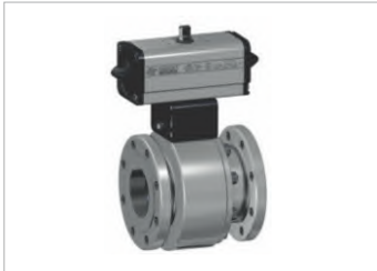
Split Body Valve with DA Actuator Material : SS / Size Range:1/2"-8" Pressure Range: PN16- 40/63-100 ANSI 150-300
