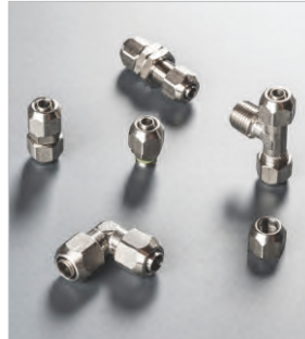
1000 SERIES Materials : Nickel Plated Brass Press.: -0,99 bar to 15 bar Temp.: NBR -20°C to +80°C | FKM -20°C to +200°C | EPDM -40°C to +160°C Fluids: COMPRESSED AIR , VACUUM , WATER , INK , LOW PRESS. FLUIDS
