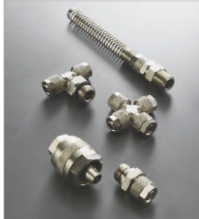
1000 SERIES Materials : Nickel Plated Brass Press.: -0,99 bar to 15 bar Temp.: NBR -20°C to +80°C | FKM -20°C to +200°C | EPDM -40°C to +160°C Fluids: COMPRESSED AIR , VACUUM , WATER , INK , LOW PRESS. FLUIDS
