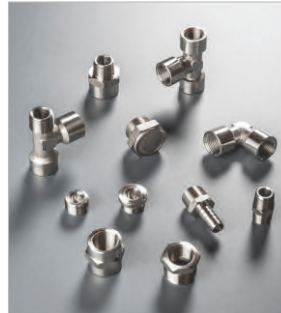
Materials: AISI 316L Temp.: -110°C to +300°C Max Press.: -0.99 to 140 bar Fluids: compressed air , water , oil Avail. Sizes : 1/8" to 1"
