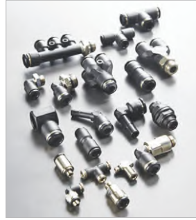
55000 Series Techno Polymeric Push-In Fittings Temp.: -20°C to +80°C Press.: -0,99 bar to 20 bar Fluids: compressed air , vacuum , water
