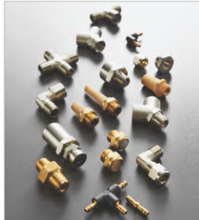
Materials: Nickel Plated Brass Press.: 150 bar Temp.: +300°C Fluids: compressed air , water , oil Avail. Sizes : 1/8" to 1"
