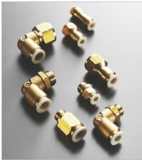
55000 Series Food & Drink Series Materials : CW510L Brass Body Temp.: -15°C to +190°C Press.: -0,99 bar to 20 bar Specially For Drinking Water Coffee Machines
