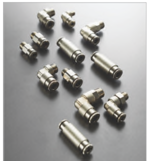
58000 Series High Pressure Push In Fittings Materials : Nickel Plated Brass Temp.: -30°C to +150°C Press.: 0 bar to 150 bar
