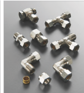
9000 Series ( Compression Fittings ) Materials: Nickel Plated Brass Max. Press.: 128.6 bar Temp.: -60°C to +300°C
