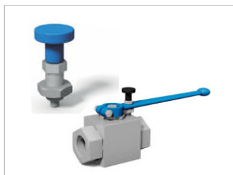
2/2 way ball valve with detents – safety against unintentional actuation. Pmax:500 bar, Size: DN4-25/40
