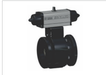
Split Body Valve with SR Actuator Material : Carbon steel / Size Range:1/2"-8" /Pressure Range: PN16- 40 / ANSI 150-300
